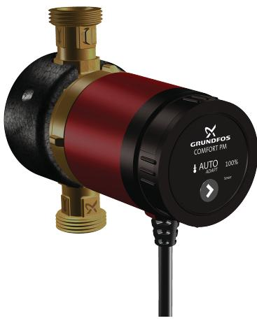
The Grundfos Comfort BA PM and BXA PM pumps are designed for recirculation of domestic hot water in single- and two-family houses securing hot water instantly to all faucets. The pumps have a corrosion-resistant pump housing suitable for drinking water and are powered by a single-phase, high-efficiency ECM with permanent-magnet rotor.
