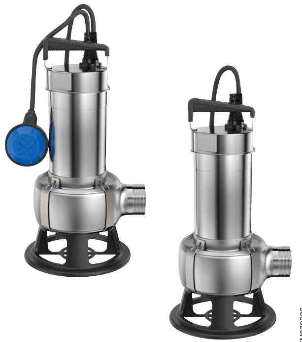
UNILIFT AP50B is a submersible pump designed for pumping effluent. The pump has a side outlet allowing easy adaptation to existing pipes including auto coupling systems. The pump is able to handle particles up to 50 mm.
