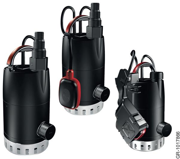
The UNILIFT CC pumps are single-stage, highly robust submersible pumps capable of pumping down to a 3 mm water level and handling particles up to 10 mm. The pump body contains a cooling jacket for operating partly submerged. The pumps have both a top and a side outlet, allowing easy adaptation to existing pipes including auto coupling systems.
