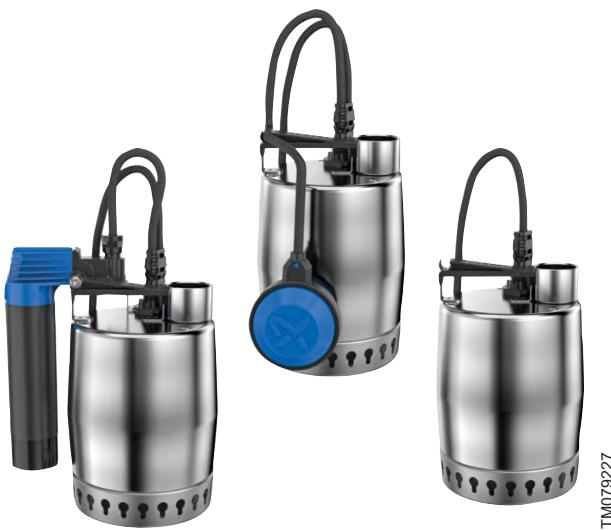
UNILIFT KP submersible, stainless-steel drainage pump in a compact design with hermetically sealed stator housing (canned motor). It has a service-friendly and sustainable product design. The pump body contains a cooling jacket for partially submerged operation. The pump is able to handle particles up to 10 mm.
